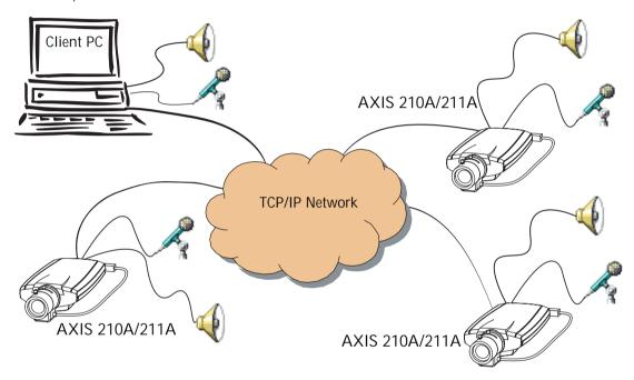
An example of a network using AXIS 210A/211A cameras to transmit audio and video across the network.
